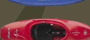
Weight range: 180-240 lbs. / 81.6kg-108.9kg Cockpit: 33.5"x19"/83.75cmx47.5cm Deck height: 13"/ 32.5 cm Boat weight: 33 lbs. /15kg Volume: 60gal/ 227.1L Width: 25.75"/ 64.4cm
