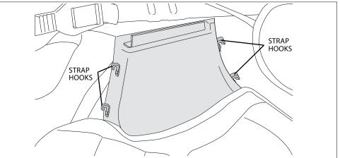
**PRO TIP** - ETHOS hip pads are designed to make the cockpit more roomy and comfortable for carrying. Ethos hip pads can be replaced with traditional Wave Sport hip pads for a tighter fit. Contact your dealer for more details.
